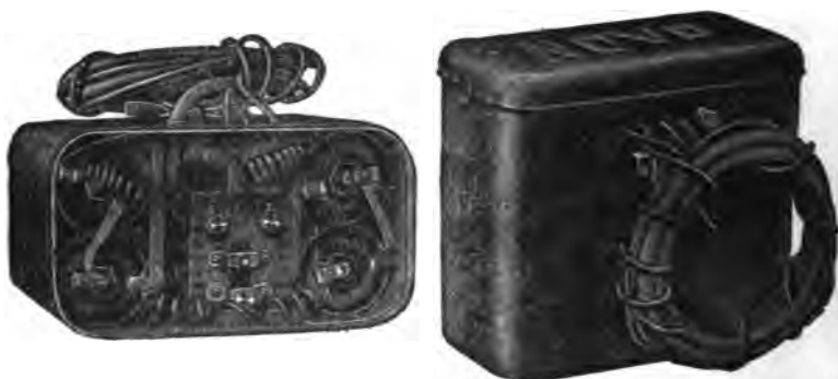
FIG. 180.—Ignition Apparatus for a Gas Engine. The illustration to the left shows the interior with four dry cells and a spark-coil. The illustration to the right shows the waterproof case, switch, and necessary wiring.
